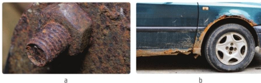
Figure 4. Corrosion (rust) of nut and bolt (a), car (b)
