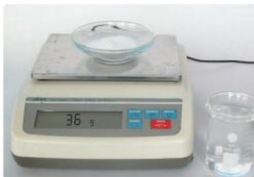
The solubility of table salt (NaCl) is 36 g/100 g of water at 20°C
