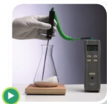
Figure 4.4 Solid barium hydroxide and solid ammonium chloride in a flask on a damp piece of wood. As the two chemicals mix, an endothermic reaction occurs causing a drop in temperature which freezes the water between the conical flask and the block of wood
