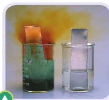
Figure 3.7 Copper reacts with nitric acid but aluminium does not
