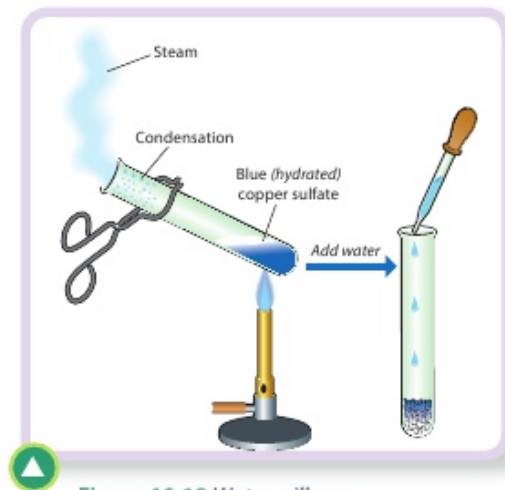
Figure 10.18 Water will cause anhydrous (dry) copper sulfate to change colour from white to blue
