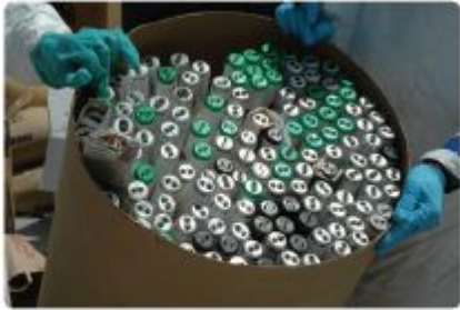
Fluorescent light tubes contains mercury
