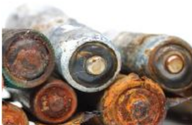
Old battery leak
