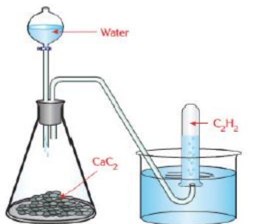
Preparation of acetylene from calcium carbide
