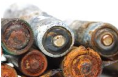
Old battery leak
