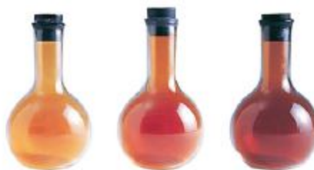
The effect of temperature. \text{NO}_2 gas has reddish-brown colour while \text{N}_2\text{O}_4 is yellow.
