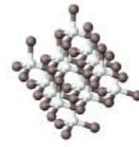
Crystal lattice of silicon carbide
