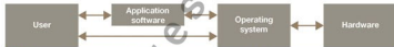
1.3 The operating system acts as a bridge between user and computer hardware
