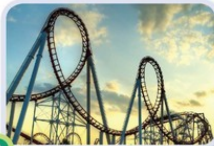
Figure 5.11 In a roller-coaster, the cars first of all climb to a great height – gaining potential energy. During the ride, this is converted first into kinetic energy as the cars fall and then back to potential energy as they climb again. This cycle is repeated over and over.
