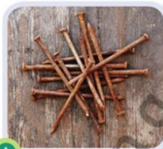
Figure 4.2 Iron is oxidised when rusting occurs
