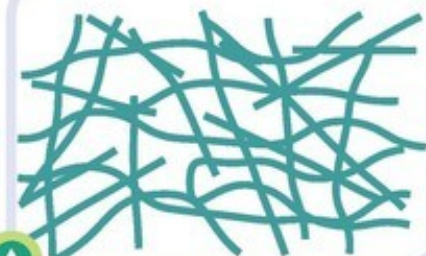
Figure 11.5 Low-density polythene: more branched chains.
