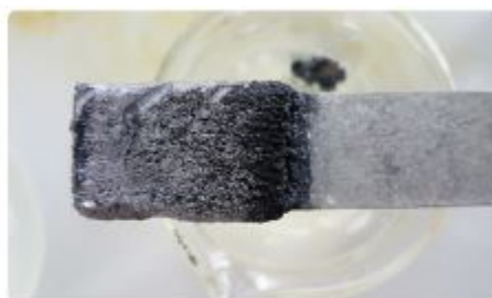
Formation of lead (Pb) on zinc (Zn) plate
