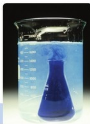
4.16 Diffusion: the dark blue solution is spreading out into the pale blue solution
