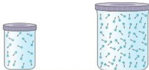
4.3 The container on the right holds more particles and therefore more heat energy
