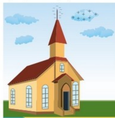
7.23 The positive charge in the air attracts a negative charge to the lightning conductor. The two neutralise each other
