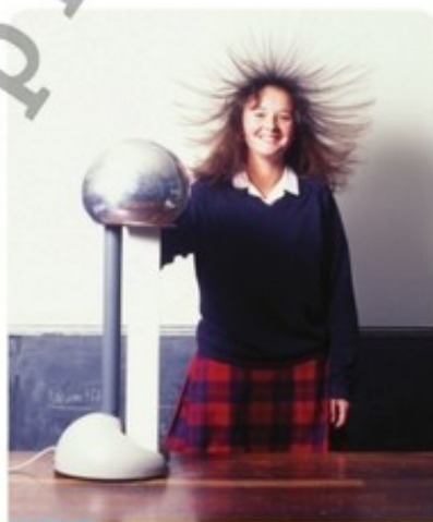
7.18 A girl placing her hand on a Van de Graaff electrostatic generator. Strands of the girl's hair repel each other because they are similarly charged
