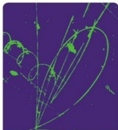
10.9 This photograph shows the tracks left when a subatomic particle decayed, creating six new particles, of various mass and charge. The different tracks represent the paths of these particles through a magnetic field
