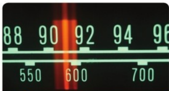
8.5 The dial of a radio showing the different stations and frequencies, which are selected using capacitors
