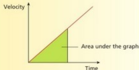
1.38 In this velocity–time graph, the slope is the acceleration. The area under the graph is the distance travelled
