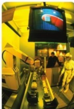
7.5 A clean room in an Intel plant, showing the protective clothing used by technicians in the manufacture of semiconductor chips
