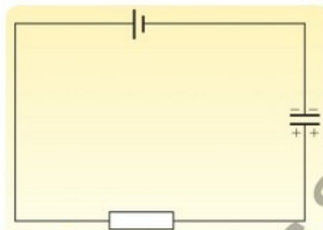
8.6 In a d.c. circuit, the current will flow only until the capacitor is charged
