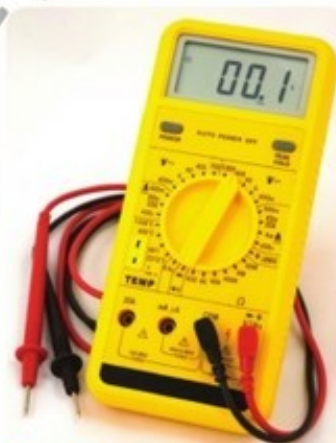
8.11 A modern multimeter which can act as a voltmeter, ammeter or ohmmeter
