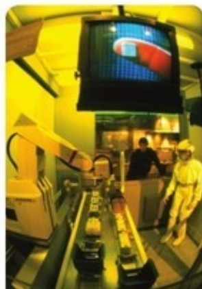
7.5 A clean room in an Intel plant, showing the protective clothing used by technicians in the manufacture of semiconductor chips
