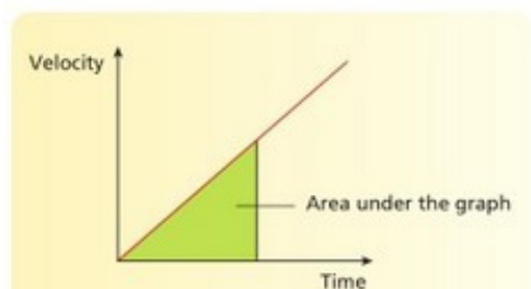
1.45 In this velocity–time graph, the slope is the acceleration. The area under the graph is the distance travelled
