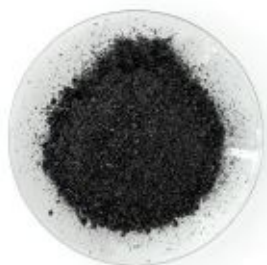
Manganese dioxide acts as a catalyst for the decomposition of hydrogen peroxide
