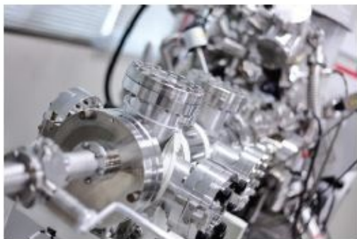
X-ray photoelectron spectrometer. X-ray structural analysis methods study the geometry of molecules.
