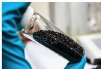
Activated carbon used as the catalyst for the catalytic synthesis of benzene
